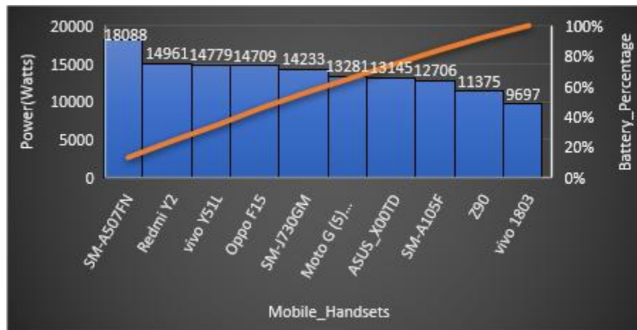
Figure 6 : Cumulative frequency graph of different handsets and their power consumption varying between the battery percentages
