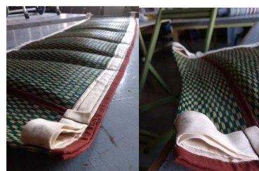
Fig 23, 24: 4 ply Muslin straps stitched on the either ends of the mat, looped at the ends.
