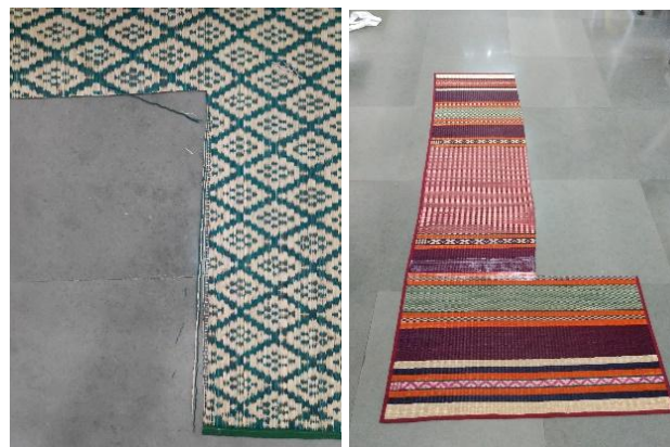
fig. 12 strands coming out of Jacquard mat in the absence of glue when a specific size was cut. fig. 13 Specific size cut out of 50 counts handloom mat.
