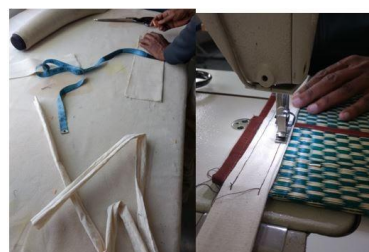
Muslin straps stitched on the either ends of the mat.
