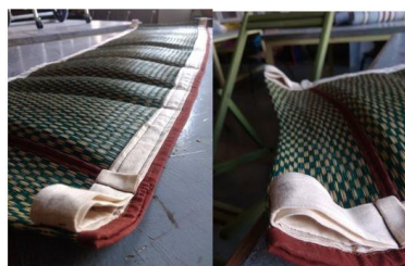
Fig 23, 24: 4 ply Muslin straps stitched on the either ends of the mat, looped at the ends.
