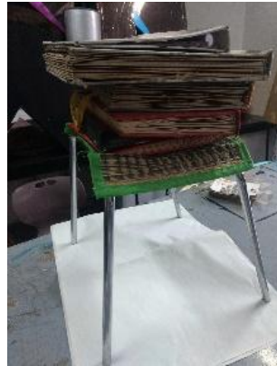
Fig. 9 (Starting on January 15, 2019 a set of books weighing about 6 kgs were kept on the surface for over 2 months, constantly.)
