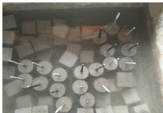
Figure (3): Specimen placed in the curing tank
