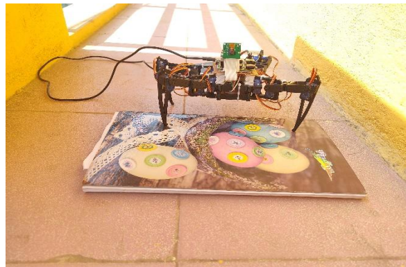
Fig 6.4: Image of Spi-bot with camera climbing uneven surface
