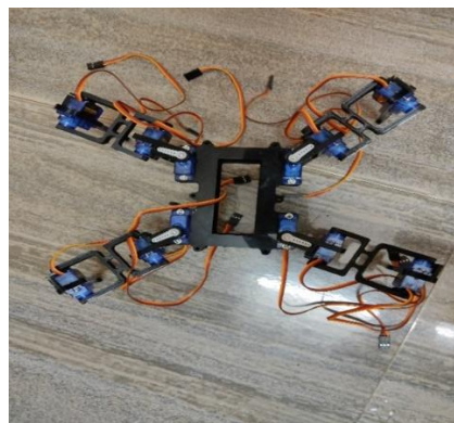
Fig 6.1: Image of the robot setup of servo motor and 3d Printed parts.
