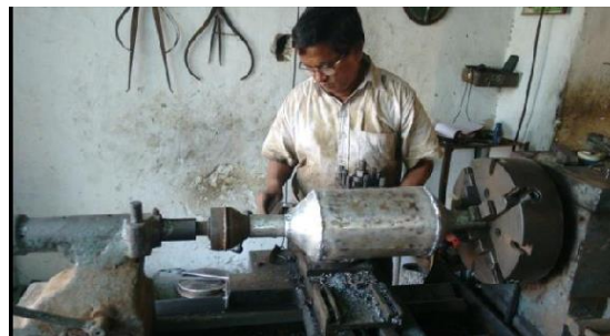
Fig7: Fabrication of catalytic convertor
