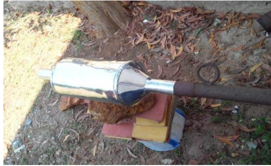
Fig8: Catalytic convertor fitted to engine exhaust
