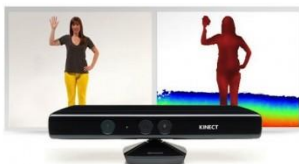
Fig.1.b. Hand gesture recognition using Kinect
