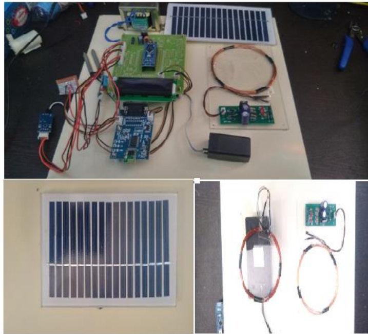
Fig 2: Wireless Power Transfer Overview, Input Source, Wireless Power Transfer Module
