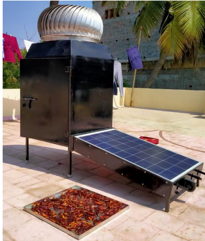
Fig. 1. Pictorialview of open sun drying and solar dryer drying on Red chilli.
