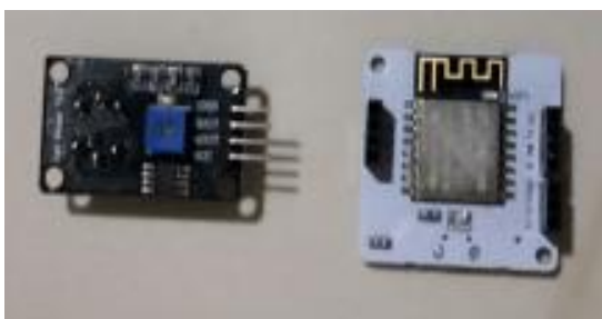
Figure 7 MQ-7 & 135 sensors with a BOLT IOT device
