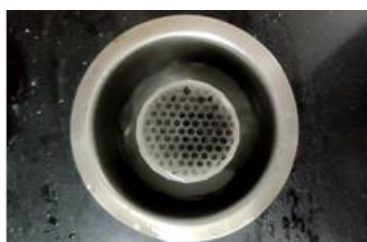
Figure 3 3-D printed activated carbon wash coated device
