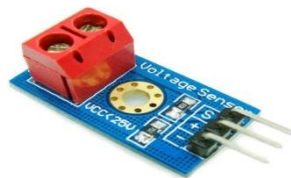
Figure 6. Voltage measuring device
